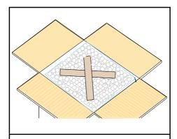
3 COMPLETELY FILL ALL REMAINING SPACE IN THE BAG WITH VERMICULITE, SEAL BAG WITH 75MM ADHESIVE TAPE.
