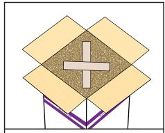
Completely fill all remaining void space around your inner packaging(s) with vermiculite - including a minimum 40mm above. Seal the poly liner bag with 75mm adhesive tape.
