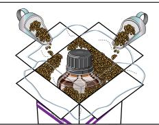
Place poly liner bag inside box and insert a minimum of 40mm vermiculite at the bottom. Place your inner packaging(s), surrounded by a minimum of 40mm vermiculite in all directions.
