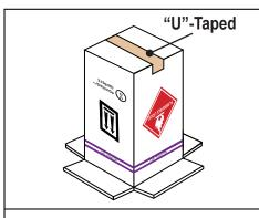
Assemble box by folding in bottoms flaps first. Seal flaps with 75mm adhesive tape in a 'U' shape
