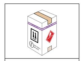
Close top flaps of box and seal closed with 75mm adhesive tape in 'U' shape
