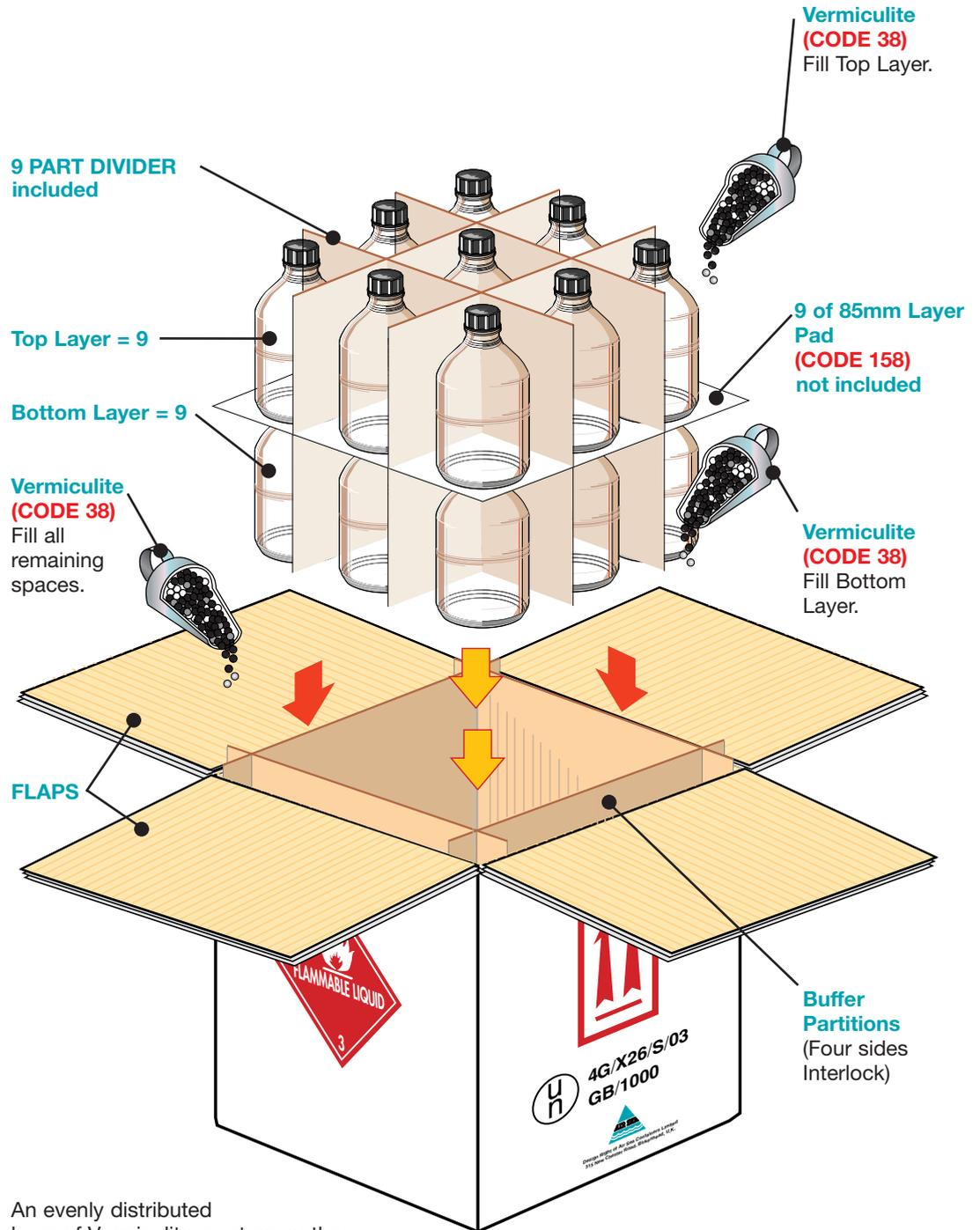
An evenly distributed layer of Vermiculite must cover the bottom and top of the packaging spaces.
