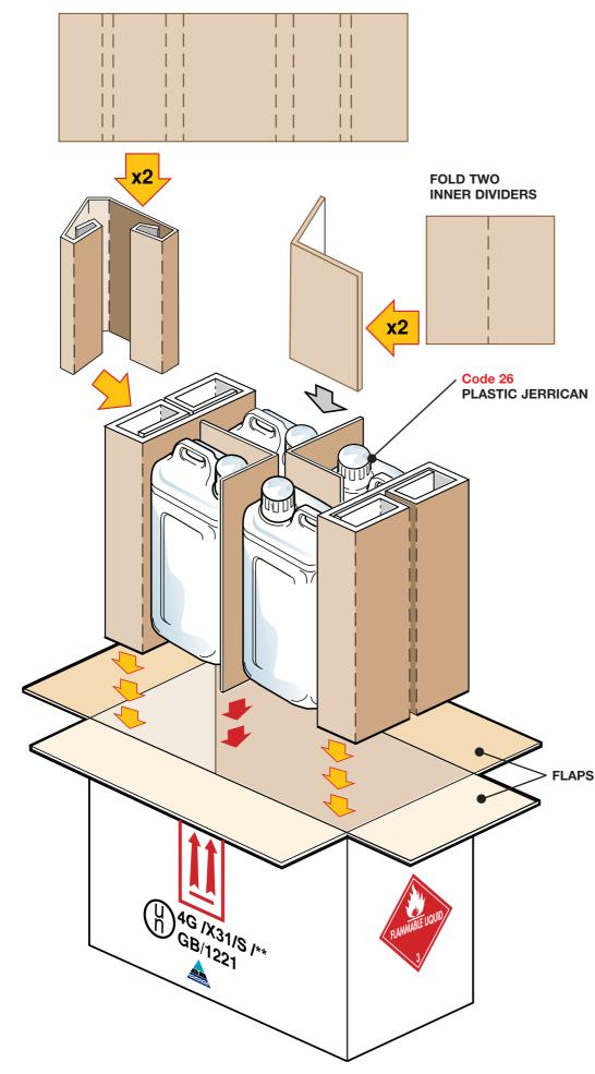
ASSEMBLY DETAILS: FIBREBOARD BOX: 4G OUTER
