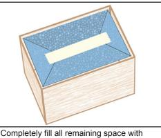
Completely fill all remaining space with vermiculite ensuring a minimum layer of 55mm vermiculite at the top of the box. Seal bag with 75mm adhesive tape.
