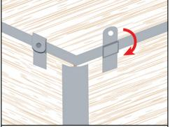
Using our special locking tab tool bend each tab into the locked position and finish off with a gentle tap. (conventional tools can also be used)
