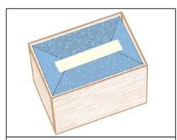
Completely fill all remaining space with vermiculite ensuring a minimum layer of 42mm vermiculite at the top of the box. Seal bag with 75mm adhesive tape.
