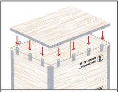
Unfold box and, ensuring all slots on base are aligned with the corresponding locking tabs, push down firmly.
