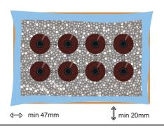
Place plastic liner bag inside box and add a minimum base layer of 42mm vermiculite before placing your inner product(s) into the box ensuring minimum spacing as shown
