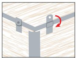
Using our special locking tab tool bend each tab into the locked position and finish off with a gentle tap. (conventional tools can also be used)
