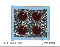
Place plastic liner bag inside box and add a minimum base layer of 35mm vermiculite before placing your inner product(s) into the box ensuring minimum spacing as shown
