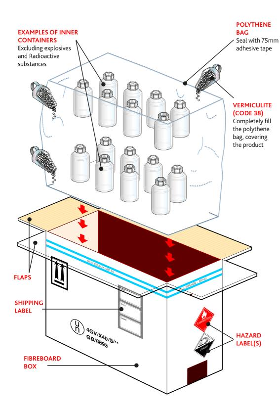
An evenly distributed layer of vermiculite must cover the bottom and top of the packaging spaces.
