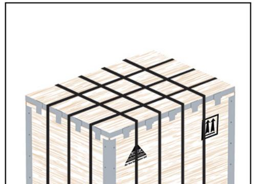
Finish by adding 15mm strapping to the box as shown.
