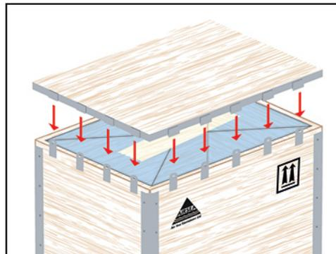
Place the lid on top of the box and lock closed as shown in steps 1 & 2.
