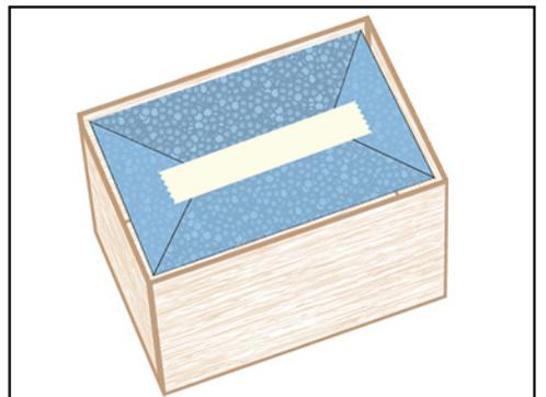
Completely fill all remaining space with vermiculite ensuring a minimum layer of 55mm vermiculite at the top of the box. Seal bag with 75mm adhesive tape.
