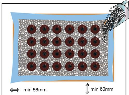
Place plastic liner bag inside box and add a minimum base layer of 55mm vermiculite before placing your inner product(s) into the box ensuring minimum spacing as shown
