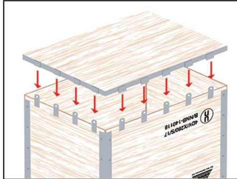
Unfold box and, ensuring all slots on base are aligned with the corresponding locking tabs, push down firmly.
