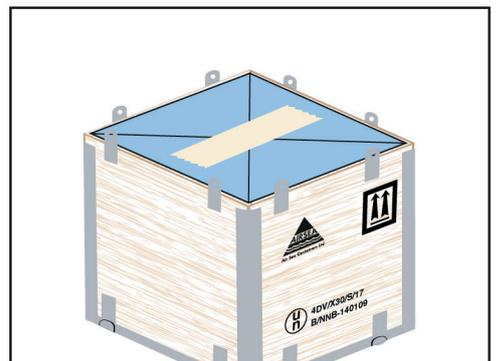
Completely fill all remaining space with vermiculite ensuring a minimum layer of 35mm vermiculite at the top of the box. Seal bag with 75mm adhesive tape.
